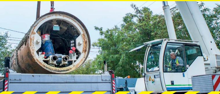
Wide range of diameters (250–3,000 mm) using upsize kit and modified cutterhead Pipe materials: reinforced concrete, GRP, polymer concrete, steel
